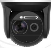
Hikvision Laser smart PTZ Dome Cameras DS-2DF8236I5W-AELW are able to capture high quality images in dim light environment with its laser IR light, which can reach up to 500m IR distance. Embedded with 1/1.9" progressive scan CMOS chip makes DWDR and 2MP real-time resolution possible. With the 36X optical zoom Day/Night lens, the camera offers more details over expansive areas.
