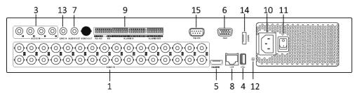
The rear panel of DS-7324HDT-I provides 24 video input interfaces.
